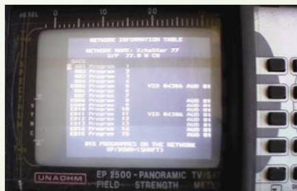
■ Diego's satellite meter shows the NIT table of one of the transponders of ECHOSTAR 6A he is receiving
