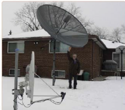
Tony Di Rienzo in his backyard standing next to his 3-meter dish. In front of him is one of his 120cm antennas with 8x8 motor.
